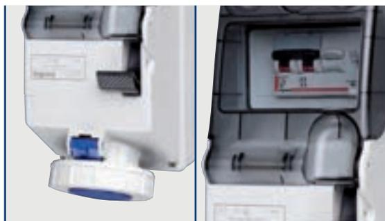
Double mechanical interlocking switch cannot be turned on unless a plug is inserted. Once switched on, the plug cannot then be removed until the switch is turned off
