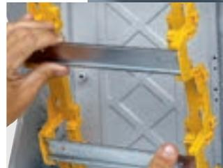
Removable chassis for wiring outside the enclosure
